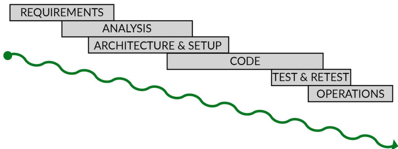
As you can see from the diagram on the previous page, all requirements gathering, planning and design work is completed before any coding takes place. Testing of developed code doesn't occur until all or most of the coding is complete, and there is no opportunity to receive feedback or generate incremental value as the project advances. In short, risk is carried throughout the duration of the project, often resulting in a product that is unproven or unfinished.
